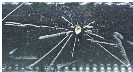
Thorite mineral in a cloud chamber. The streaks are 'clouds', nucleated by radiation
