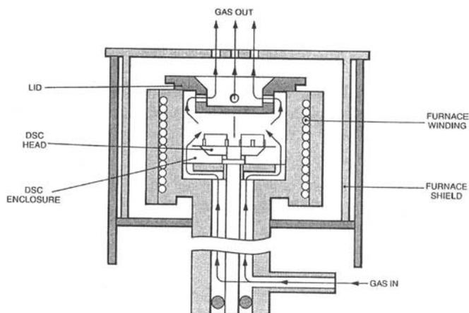
Samples and reference materials in pans sit on plates, which are in thermal contact with thermocouples. These are enclosed by a furnace, which enables heating/cooling of both. The heating/cooling can be controlled via a third thermocouple or the thermocouple of the reference material.
