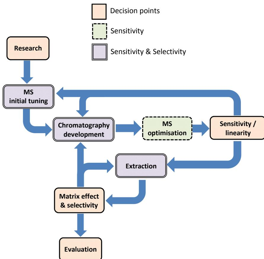
Figure 3.1: Stepwise optimisation of the overall LC-MS method
