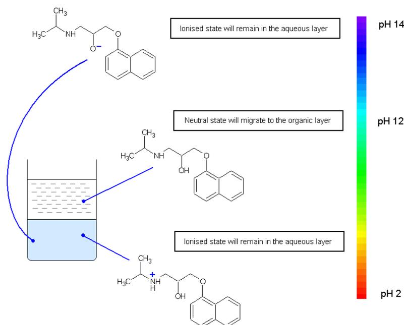
Figure 4.2: Illustration of how solution based chemistry may be manipulated using pH to encourage partition of propranolol ( $\text{pK}_a = 9.5$ )[18] into aqueous or organic liquid phases.
