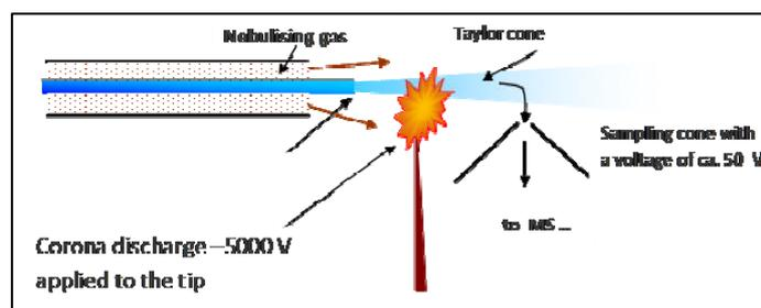
Figure 2.4: Schematic of APCI source
