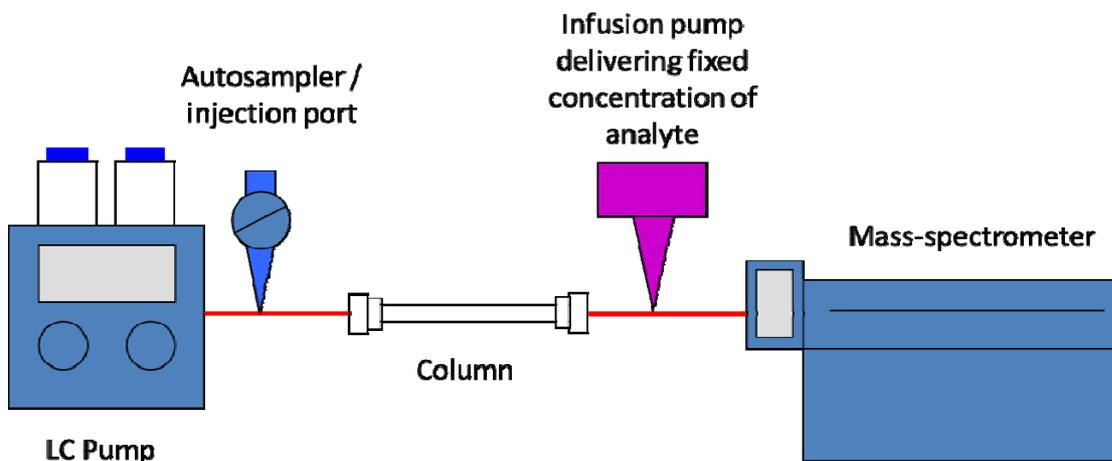
Figure 3.2: Use of post-column infusion for assessment of matrix effects
