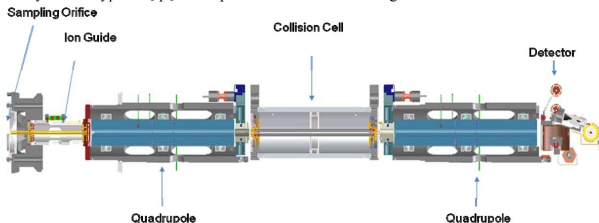
Figure 2.2: Schematic view of a typical triple quadrupole (QqQ) mass spectrometer
