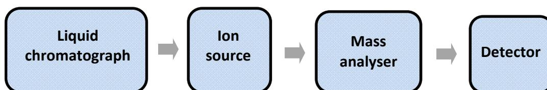
Figure 2.1: Basic components of an LC-MS system
