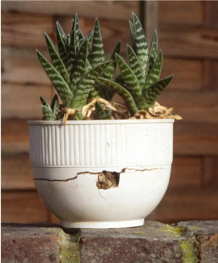
Filled HDPE pot after 24 months indoor exposure (W-facing window)
