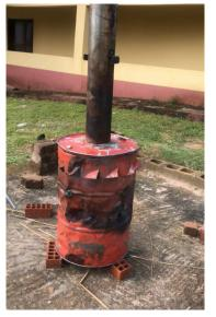
Figure 2. Picture of a pyrolysis kiln, locally made in Nigeria, from an oil barrel.
