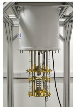
A Cryostat, where liquid helium is used as a coolant and gold plating shields sensitive samples from radiation. Photo credits Andrew Guthrie.
