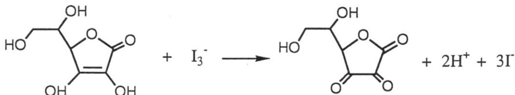
An excess of iodine is generated in situ from a standard solution of potassium iodate, after the addition of an excess of potassium iodide. After reaction the excess iodine is determined by titration with a standard solution of sodium thiosulfate, using Thyodene as the indicator.
