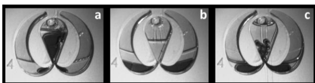
Figure 5. a Loading of oil (transparent phase) and water (dark phase). b Compression of the liquids while spinning. c Formation of water droplets with the backing down of the liquids at low rpm.
