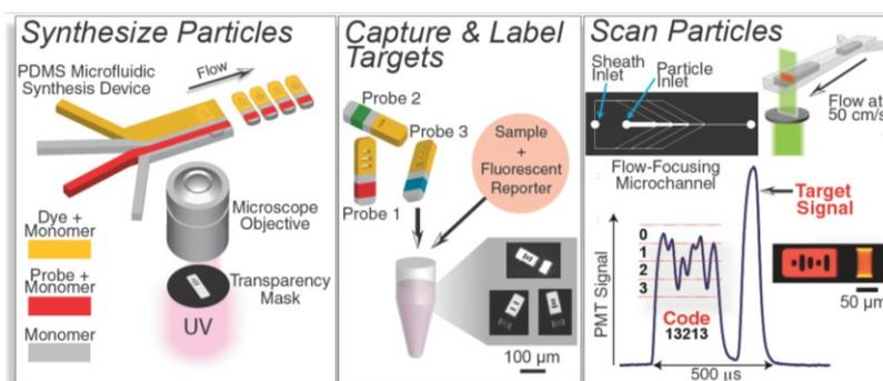
Figure 1: Gel particles are simultaneously synthesized, encoded, and functionalized via stop-flow lithography in a PDMS microfluidic device. For multiplexing, each particle has a fluorescently-doped graphical barcode that corresponds to the identity of the probe(s) covalently immobilized in a separate region. Codes and target levels can be rapidly read in a microfluidic scanning device at a rate of 25 particles/s.
