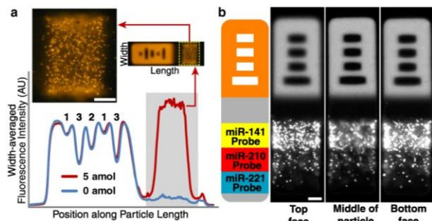
**Figure 3: Single-molecule reporting resolution for miRNA analysis.** (a) Overlaid stationary scans of particles exposed to either 0 or 5 amol of miR-210, with magnified color image of top face of probe region. Each fluorescent spot represents a single target-binding event. (b) Multi-probe particle exposed to solution containing 5 amol miR-141, 1 amol miR-210, and 0.2 amol miR-221. All scale bars are 20  $\mu\text{m}$ .
