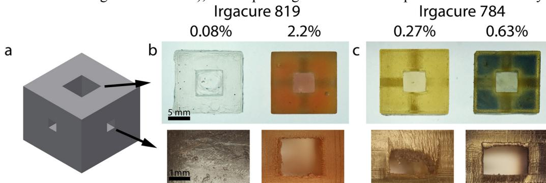
*Figure 1: 3D-printed PEG-DA cubes. (a) Design of the cube. Arrows indicate where the pictures were taken. (b) Cubes printed with PEG-DA/I819. Top row shows the surface of the cube with square well and bottom row a photograph of one square channel of the walls. (c) Cubes printed with PEG-DA/I784. Scale bar is the same for each row.*
