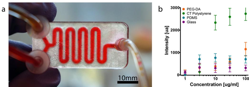
Figure 2: (a) 3D-printed microfluidic device filled with dye. The photograph was taken ~24 hrs. after the device was filled. (b) Chart of protein adsorption tests showing the concentration of BSA-tetramethylrhodamine vs intensity of fluorescence for each material.
