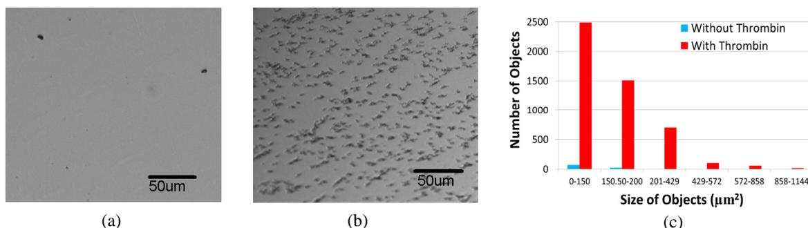
Figure 3: Scanned images of the samples with oCelloScope (a) without thrombin (no clustering) and (b) with 900 nM thrombin (high degree of clustering). (c) Histogram of the number of scanned objects vs. their size (area). The solution with 900 nM thrombin indicates a large number of objects with much higher area value - indicating numerous clusters.
