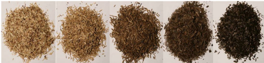
Figure 1 The change in colour of the biomass, from untreated (or raw) to biomass torrefied at increasingly higher temperatures and or residence times.
