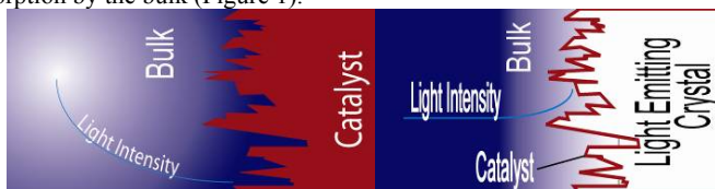
Figure 1. Graphical representation of a) Traditional photocatalytic approach, b) The local luminescent approach.
