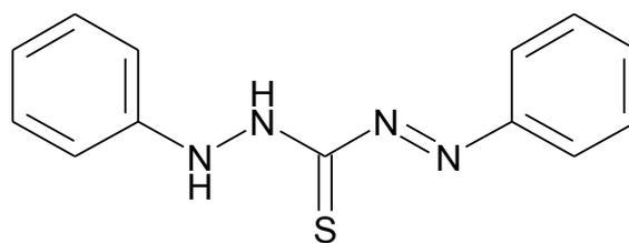
*A good analytical reagent for a metal ion should form a very strong complex with the metal ion of interest but also be very specific, that is not react with any other metal ions in solution. Dithizone is such a reagent, which is reasonably specific for  $Pb^{2+}$  forming a red complex. The colour can be used to determine the concentration of the lead (II) ions. See below for explanation of spectroscopy.*
