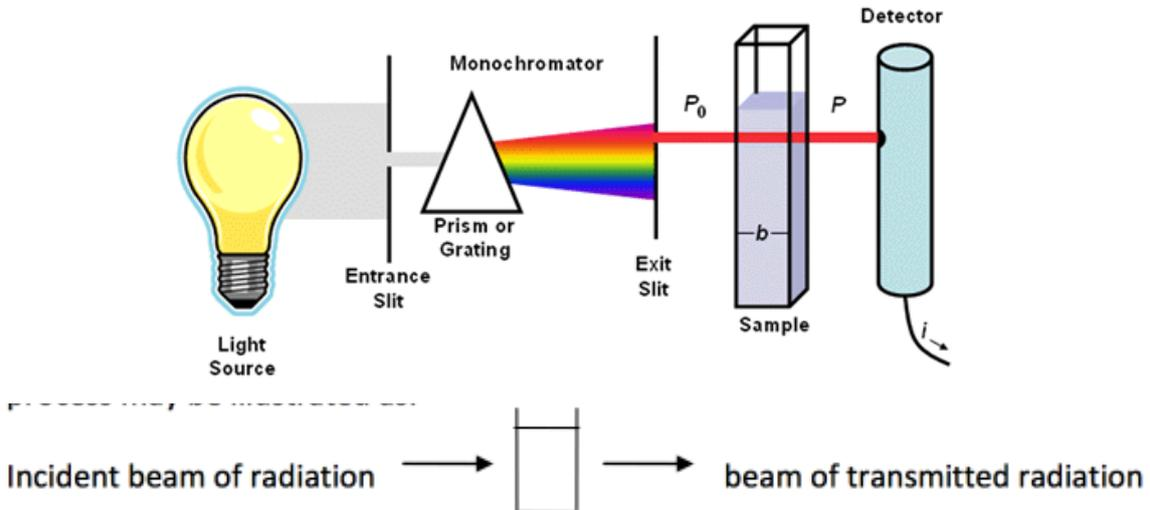
$$\text{Absorbance} = \log \frac{\text{intensity of incident radiation}}{\text{intensity of transmitted radiation}} = abc$$
