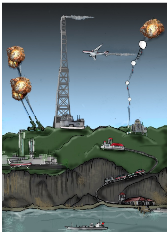
Figure 1. Proposed methods of stratospheric aerosol injection. A mountain top location would require less energy for lofting to stratosphere. Drawing by Brian West. Reprinted with permission from (5).
