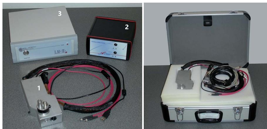
Fig. 2 Main subunits of a custom-built mobile LIBS spectrometer (left) and the instrument in a carrying case (right).
