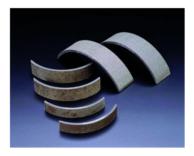
Brake linings contain phenolic resin binder, clay and powder fillers, graphite lubricants, and metallic fibers (Ba, Ca, Ti, Cu, Mg, Cr, Sb, Zn, Zr)
