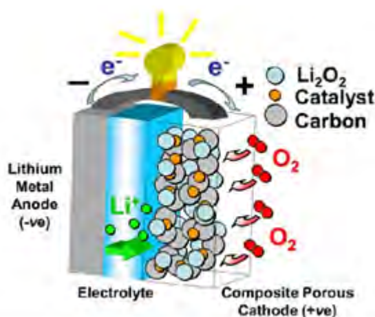
Schematic representation of a rechargeable Li-O 2 battery.
