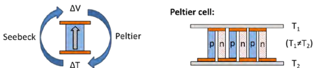
Fig. 1 Left: For a material with two junctions the Seebeck effect is defined as the voltage generated ( \Delta V ) due to a temperature difference ( \Delta T ), whereas the Peltier effect is the reverse process. Right: Schematic of a standard Peltier cell where p- and n-type pillars of material are connected electrically in series and thermally in parallel.
