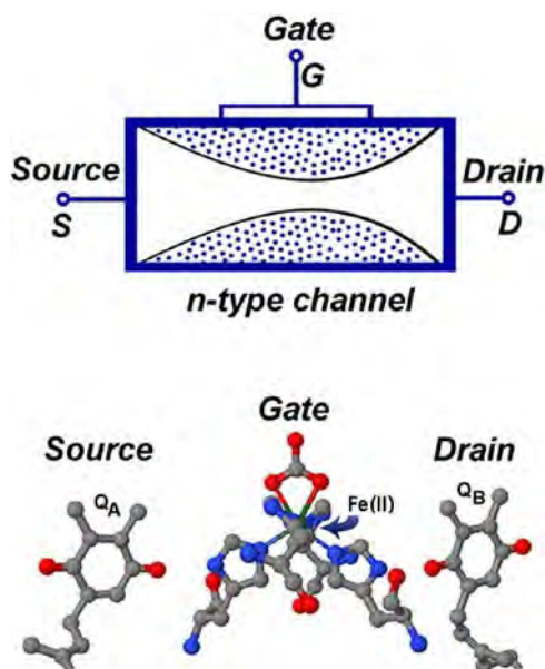
Fig.1. Comparison of a JFET (top) with the newly-discovered single molecule transistor in PSII (bottom). Both are three-terminal devices, consisting of a source, a gate, and a drain. Top: The JFET uses an electric field to “gate” the conduction of electrons between source and drain. Bottom: The single molecule transistor (an Fe(II) ion) uses the bicarbonate ligand field to “gate” the superexchange of electrons between the quinones Q A and Q B .
