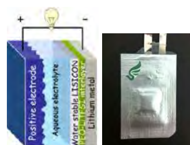
Fig. 1 (left) Schematic representation of the aqueous hybrid EC using multi-layered Li electrode and (right) AdHiCap prototype cell.
