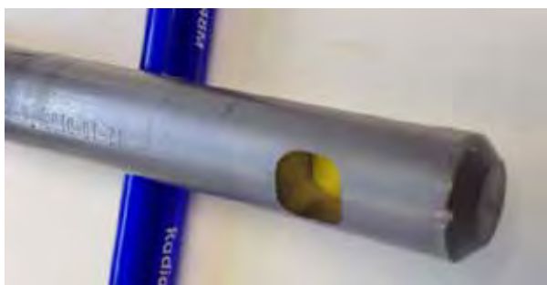
Fig. 1 Photograph of a stainless steel NanoFlex™ electrode holder after being dropped from a 1 st floor window. The electrode still gave high quality electrochemistry after drop.
