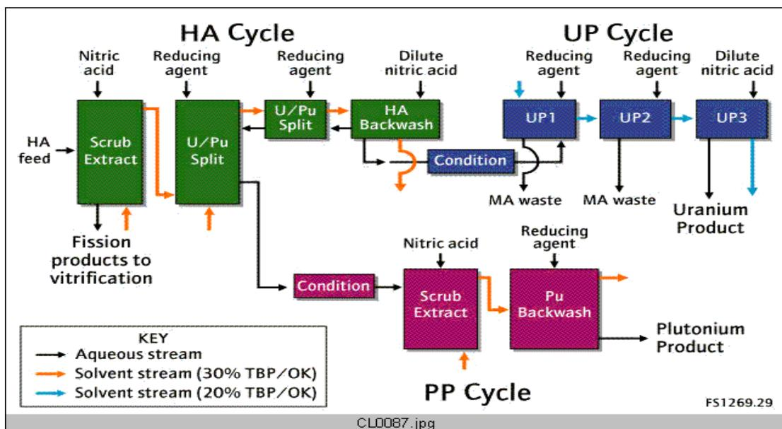
At least 96% of the weight of fuel entering the reprocessing plant is recovered as uranium which can then be recycled and used as new fuel. Up to 1% is recovered as plutonium which can then be used as mixed oxide fuel. About 3% of the fuel is waste which is vitrified in glass. This waste contains 95% of the radioactivity.
