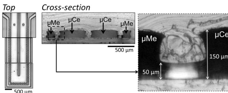
Figure 2. Top and cross-sectional views of the developed microdevice.
