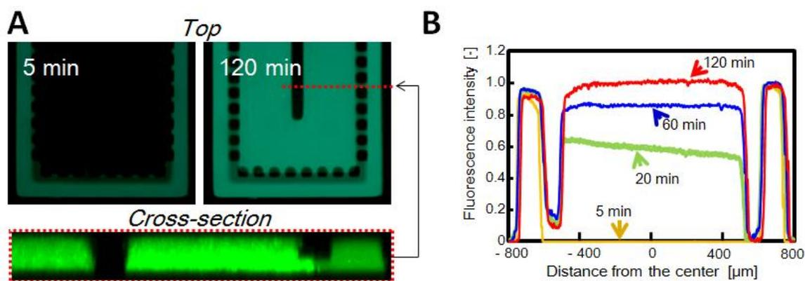
Figure 4. Introduction of the FITC labeled albumin solution into the  $\mu$ Me of the device with collagen gel in the  $\mu$ Ce. The albumin was diffused throughout the gel within 120 min (A and B).
