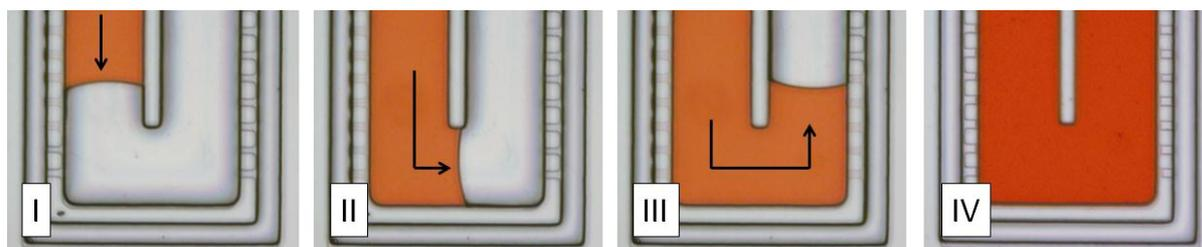
Figure 3. Introduction of the colored solution into the  $\mu$ Ce. No leakage was observed to the  $\mu$ Me.
