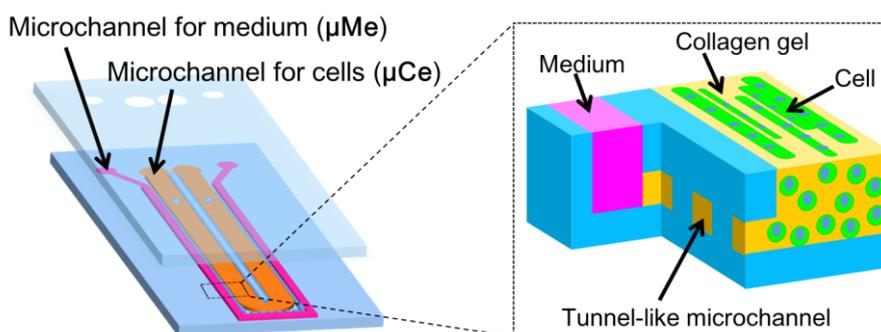
Figure 1: Conceptual illustrations of the device.
