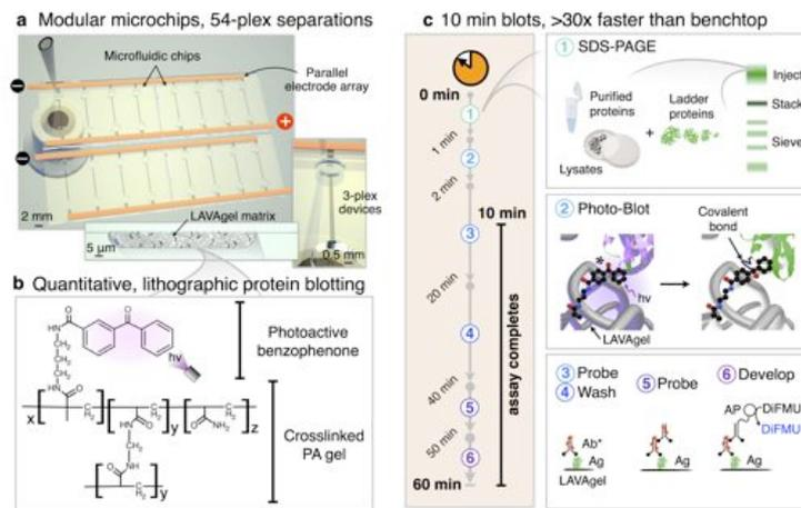
Figure 1: Micro-Western workflow in a parallelized glass chip with functional PACTgel protein capture matrix.
