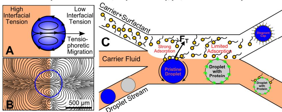
**Fig. 1:** Concept of label-free sorting using tensiophoresis. (A) Droplet migration in an IFT gradient. (B) CFD simulation. (C) Schematic of chip used for sorting droplets based on chemical contents.
