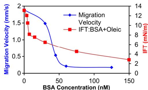
**Fig. 5:** Droplet migration velocity as a function of protein content within the droplet (Blue) and interfacial tension vs. protein concentration measured using a traditional pendant drop method (Red).
