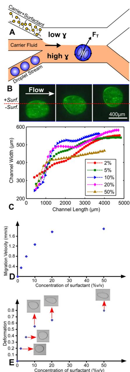
**Fig. 2: Capillary migration of droplets in a binary IFT gradient.** (A) Chip schematic. (B) Fluorescent image of migrating droplet. (C) Droplet trajectories at various surfactant concentrations. (D) Migration velocity and (E) droplet deformation at various surfactant concentrations.
