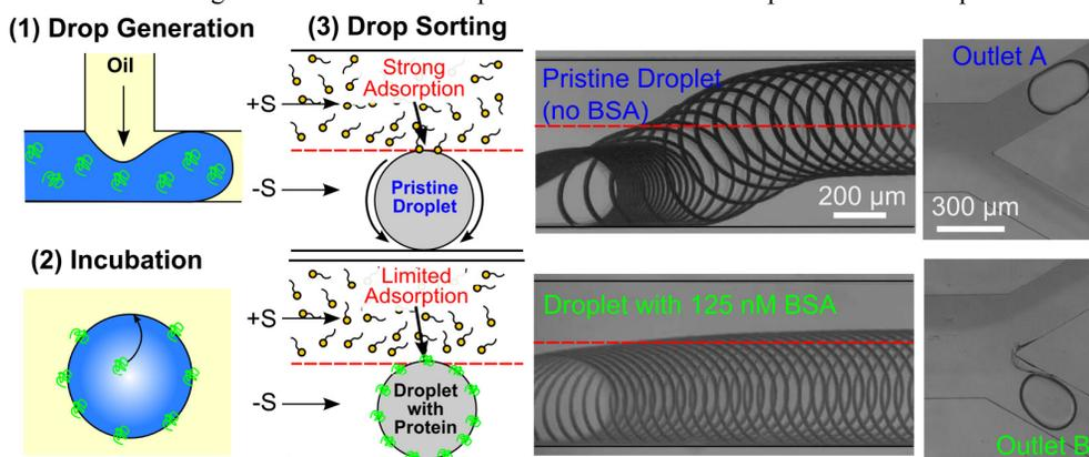
**Fig 4:** Label free droplet sorting by protein concentration. Protein sorting is accomplished in 3 steps (drop generation, incubation, and sorting). The images show the migration profile of a pristine droplet (top) versus a droplet containing 125 nM BSA in a binary surfactant profile. The migration velocity is measured near the inlet using image processing software. The two types of droplets are sorted into respective outlets A and B.
