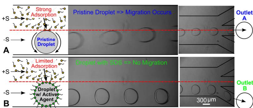
**Fig.3:** Label-free droplet sorting by chemical composition. (A) Pure droplets migrate steadily and collect at outlet A. (B) Droplet containing SDS (2.3mM) do not migrate and are sorted to outlet B.
