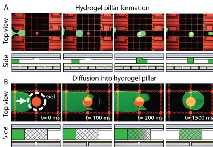
**Figure 2: Digital microfluidics for hydrogel microgel formation.** (A) Top view (stereomicroscopy) and side view (schematic) of passive dispensing mechanism in the formation of microgels. (B) Top and side views of FITC-Dextran (4 kDa) into microgel.
