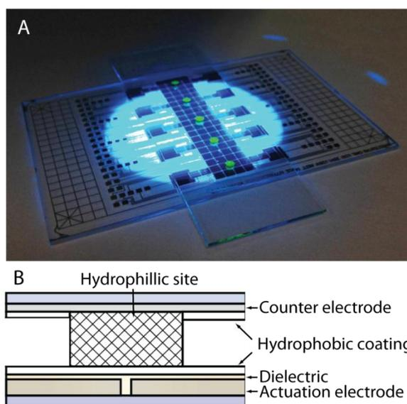
*Figure 1: Digital microfluidic device. (A) Photograph of device on stereomicroscope with five independently addressable fluorescently labelled hydrogel pillars. (B) Cross-sectional schematic of DMF device geometry.*
