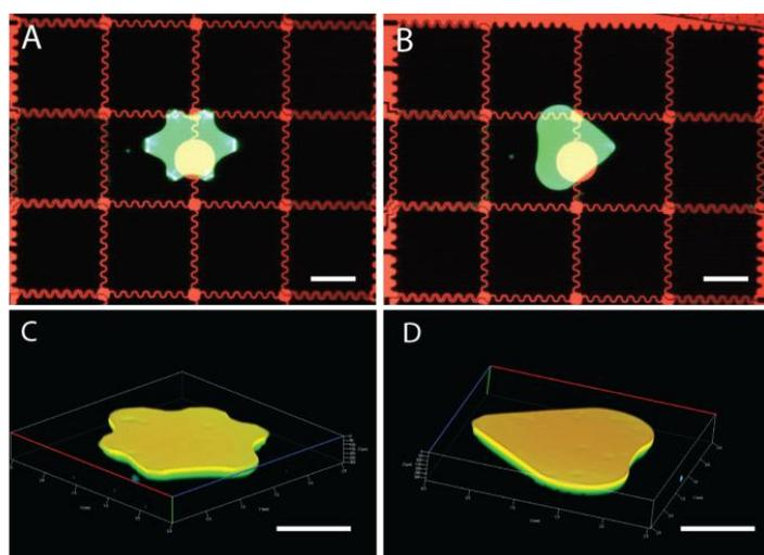
**Figure 3: DMF hydrogel geometries.** Multiple geometries can be formed by modifying the design of the patterned region on the device top-plate. (A,B) Stereomicroscope images and (C,D) confocal microscope images of star-shaped and heart-shaped hydrogel pillars. Scale bars = 1 mm.
