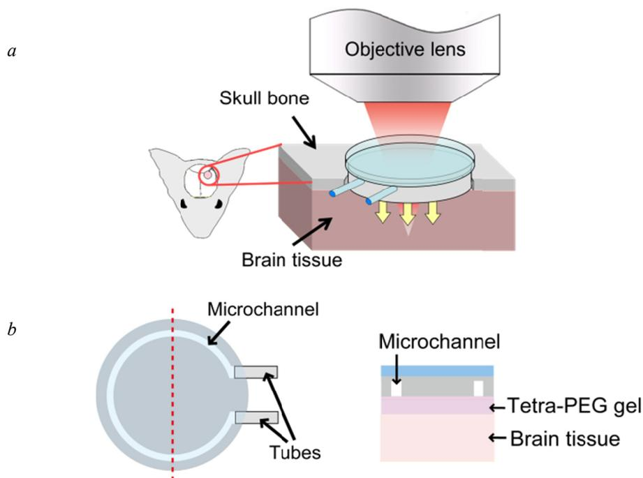
Figure 1. Brain interface device with a permeable hydrogel membrane. (a) Schematic of the microfluidic interface device mounted on a mouse skull. (b) Schematic of a microchannel in the device.
