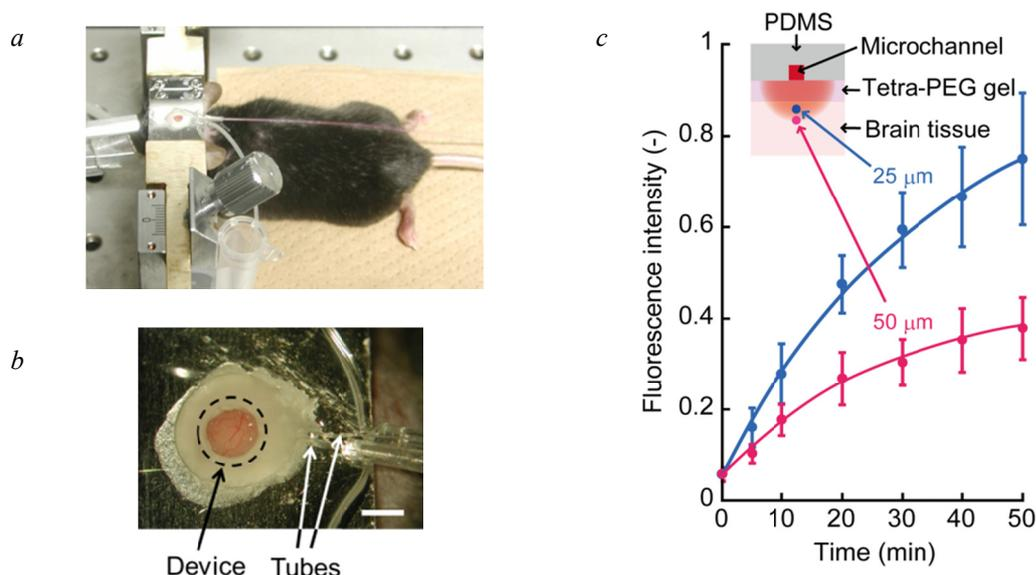
Figure 5. (a) A living mouse immobilized with the headgear. Teflon tubes were connected to the device tubes to inject solutions into the microchannels. (b) Device in the headgear. Scale bar:  $2\ \text{mm}$ . (c) Diffusive transfer of fluorescent substance in brain tissues at depths of  $25\ \mu\text{m}$  and  $50\ \mu\text{m}$ . Error bars show the standard deviations.
