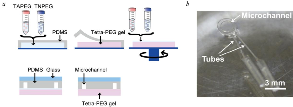
Figure 2. (a) Fabrication process of the device. PDMS with microchannels was sealed with Tetra-PEG gel. (b) Photograph of the microfluidic interface device. The device is immersed in water to avoid the deformation of the hydrogel. The device is 2.7 mm in diameter and 500  $\mu\text{m}$  in thickness.
