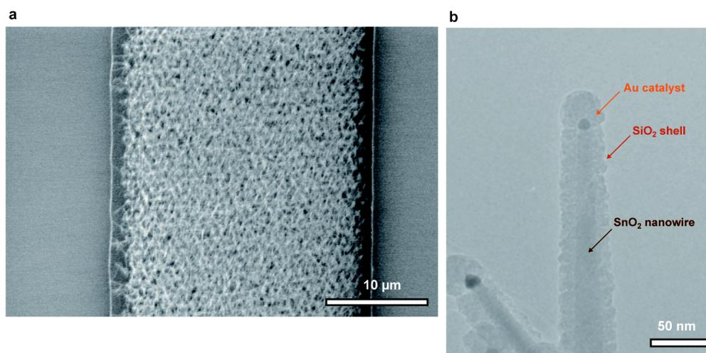
Figure 2. (a) FESEM image of fabricated nanowire array; scale bar, 10  $\mu\text{m}$ . (b) TEM image of fabricated nanowires; scale bar, 50 nm.
