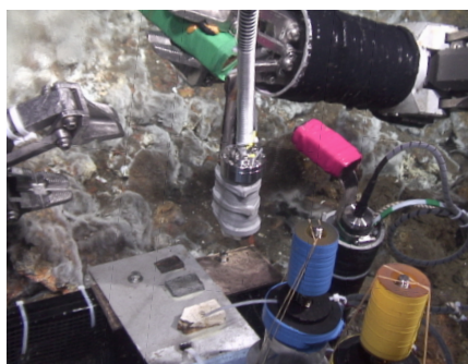
Testing of underwater LIBS at sea showing (left) the direct optic setup, (center) the fiber optic setup, and (right) an example of spectroscopic measurements made during the sea trials
