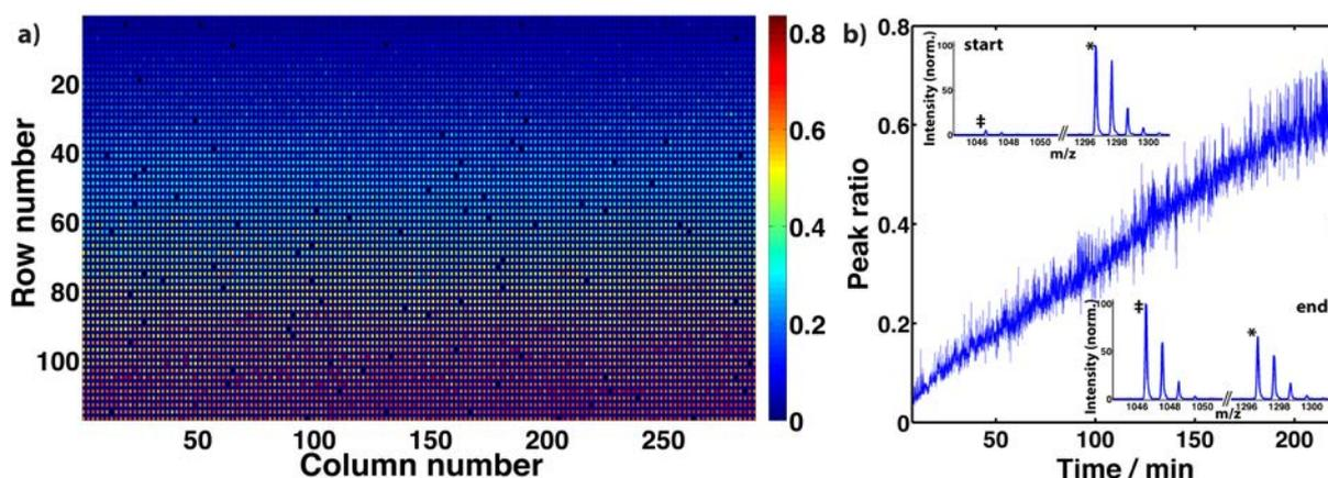
Figure 3. a) Heat map showing the progress of the enzymatic conversion in form of the peak ratio for the 8000 droplets spotted on individual hydrophilic spots and measured by MALDI-MS. b) The peak ratio as a function of time. Insets: MALDI-MS spectra from the beginning and at the end of the enzymatic reaction (\* Angiotensin I, substrate; ‡ Angiotensin II, product).
