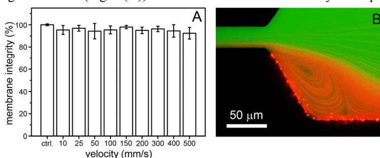
Figure 2. STE velocity impact on membrane integrity (A). Vortex produced by inertial effects using a STE velocity of 500 mm/s (B).
