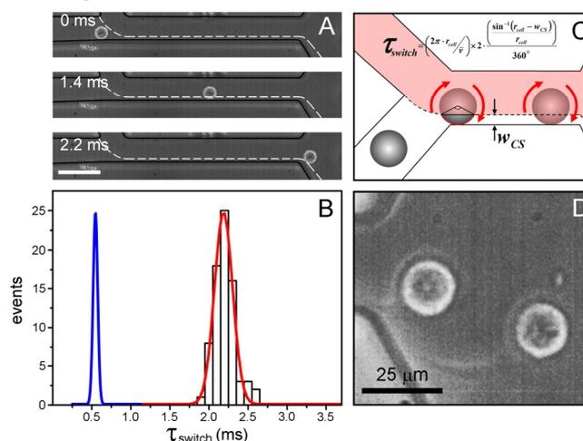
Figure 3. Cell transported through the STE (A). The  $\tau_{\text{switch}}$  for cell stimulation (red) and reaction arrest (blue) (B). Cell rolling in the STE which produces a self-mixing phenomena. The rolling  $\tau_{\text{switch}}$  is determined by the cell stream width ( $w_{\text{CS}}$ ) and the cell radius ( $r_{\text{cell}}$ )(C). Disruption of a dye-doped laminar stream by rolling single cells (D).
