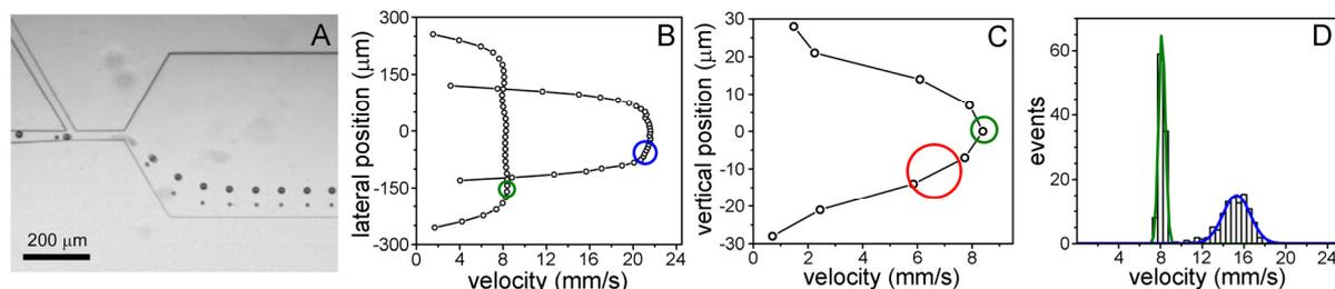
Figure 4. Size-dependent trajectories (A). Lateral (B) and vertical (C) flow profiles measured by  $\mu\text{PIV}$ . Blue, green and red circles indicate the cell positions. Cell velocity distribution in the original (blue) and optimized (green) systems (D).
