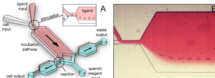
Figure 1. Diagram of the deterministic lateral displacement system with a STE for stimulation, incubation path and channel bifurcation with a STE for reaction arrest (A). Single cell deflection into a dye-doped ligand stream (B).
