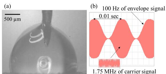
Figure 5. (a) Overlaid high-speed camera images of droplet oscillation;  $5 \mu\text{l}$  NaCl ( $\sigma = 1413 \mu\text{S}/\text{cm}$ ) droplet oscillation is synchronized with the envelope frequency. (b) AM signal is wirelessly transmitted to the EWOD electrode to oscillate the droplet. The signal is measured at the receiver. The envelope frequency is 100 Hz, and the carrier frequency is 1.75 MHz.
