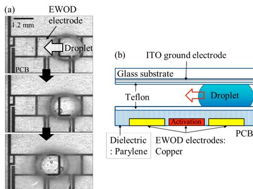
Figure 6. (a) Snapshots of NaCl droplet ( $2.5 \mu\text{l}$ ) transportation (one-step left) by shifting application of wirelessly transmitted signal from one electrode to another. The driving signal is AM as shown in Fig. 5 (except the envelope frequency = 10 Hz). (b) Cross-sectional view of droplet transportation configuration.
