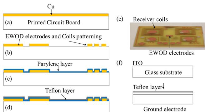
Figure 2. Microfabrication process of wireless EWOD device: (a) Cu layer ( $15 \mu\text{m}$ ) on top of  $1.5 \text{ mm}$  of PCB; (b) patterning of receiver coils (width  $50 \mu\text{m}$  and spacing  $70 \mu\text{m}$ ) and EWOD electrodes; (c) depositing of  $3.1 \mu\text{m}$  parylene layer; (d) coating of hydrophobic Teflon layer; (e) photo of microfabricated wireless EWOD chip. (f) ITO cover glass coated with Teflon for ground electrode.
