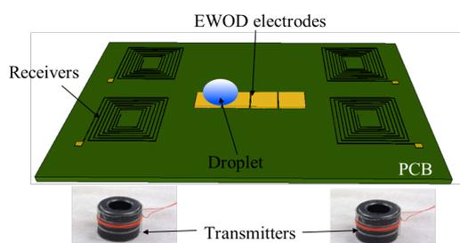
Figure 1. Integrated planar receivers with EWOD array electrodes on PCB (upper plate,  $7.5 \times 6 \times 0.15 \text{ cm}^3$ ). Each receiver coil has a rectangular shape (outer dimension  $< 2.3 \text{ cm}$ ) and center-to-center aligned with spool type transmitter coils (bottom).
