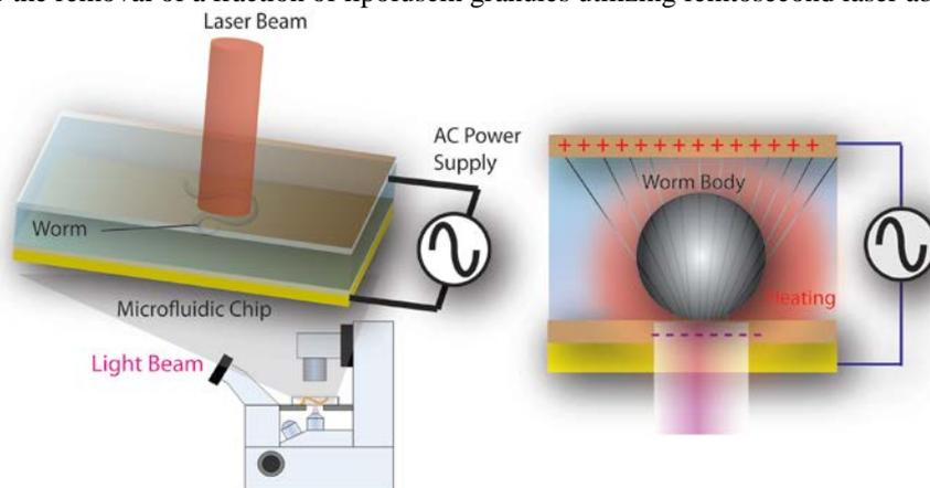
Figure 1. Schematic of the setup (left) and the electric field in an aLINK microchip under irradiation of a laser beam (right).
