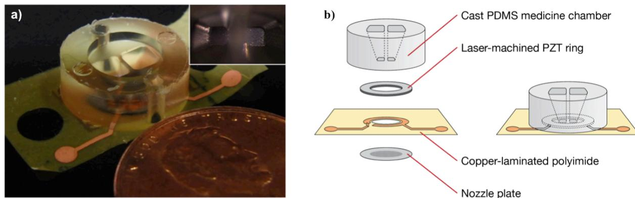
Figure 1: a) Vibrating mesh nebulizer with dual medication chamber. The volume of each medication chamber is  $9 \mu\text{L}$ . The insert shows the nozzle plate at the bottom of the chambers, which are separated by  $400 \mu\text{m}$ . b) Exploded view and schematic diagram of the nebulizer.
