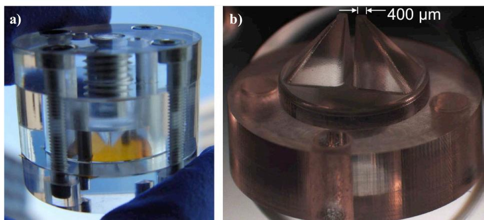
Figure 2: a) Mold for casting the dual elastomeric medication chamber on top of the nozzle plate. b) The mold insert with two half-pyramid shapes used to form the medication chambers.
