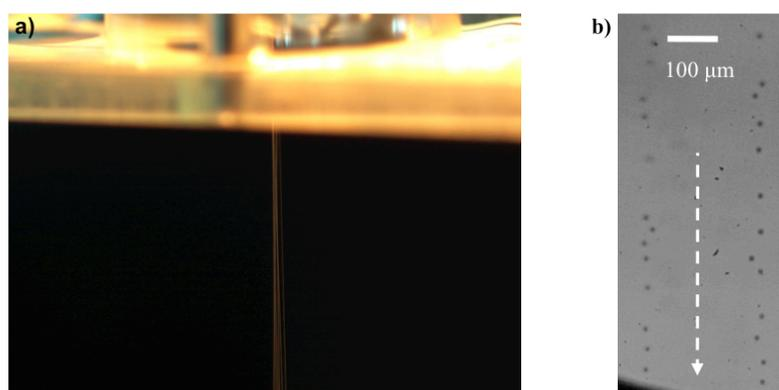
Figure 3: a) Streams of aerosol ejected from a nebulizer with a medication chamber. b) High-speed camera imaging of aerosol exiting the nozzles. Two streams of droplets are visible on both sides of the arrow. The droplets are  $\sim 10 \mu\text{m}$  in diameter. Average spatial separation between the droplets is  $\sim 50 \mu\text{m}$ .
