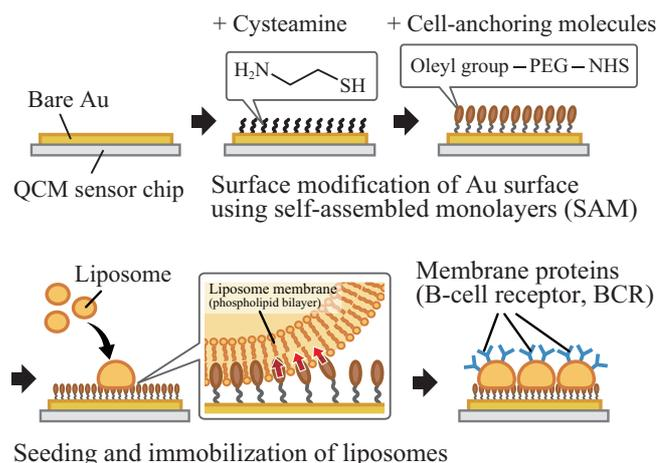
Figure 4. Liposome immobilization on the Au electrode of a QCM sensor.
