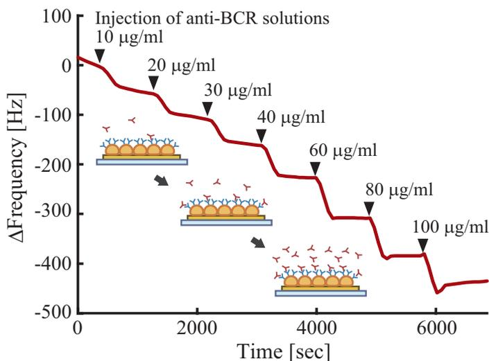
Figure 6. Frequency reduction in response to different concentrations of anti-BCR solutions.
