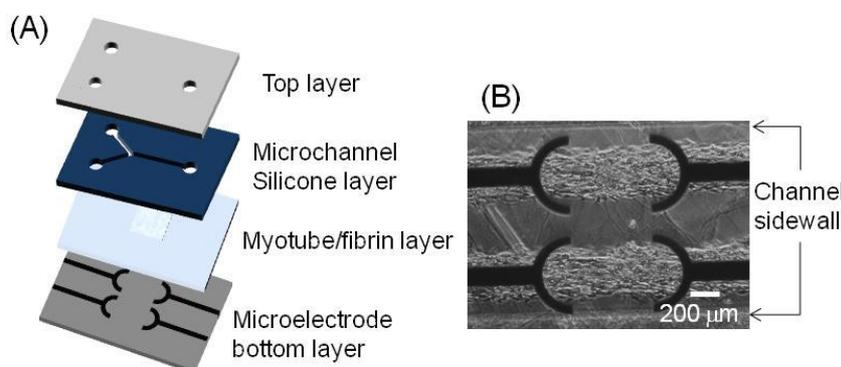
Figure 4. (A) Structure of the myotubes/microelectrode gel sheet combined with the microfluidic channel. (B) Phase-contrast micrograph of the myotube line patterns in the microchannel.
