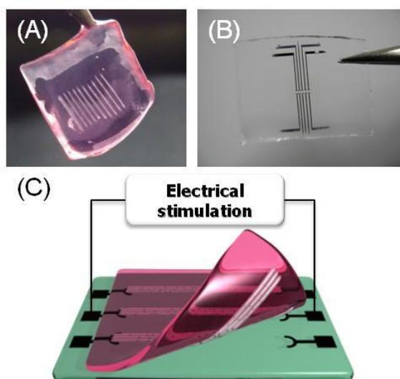
Figure 1. (A, B) Photograph of a fibrin gel with myotube line patterns (A) and a conducting polymer PEDOT-printed hydrogel (B). (C) Myotube/fibrin gel combined with the PEDOT microelectrode-printed hydrogel sheet.
