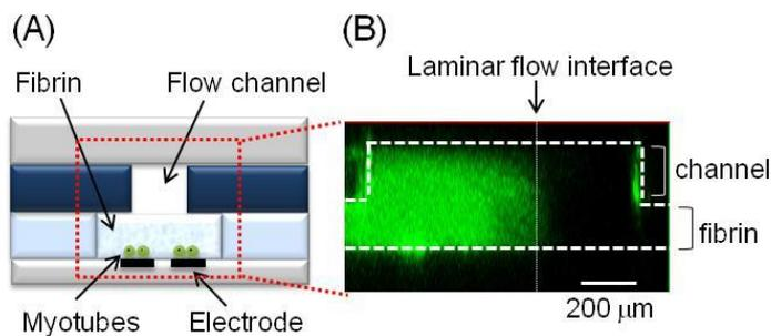
Figure 5. (A) Illustration of the device cross-section. (B) Fluorescent micrograph of the device cross-section when two-phase laminar flow of fluorescein solution and water was formed in the microchannel.
