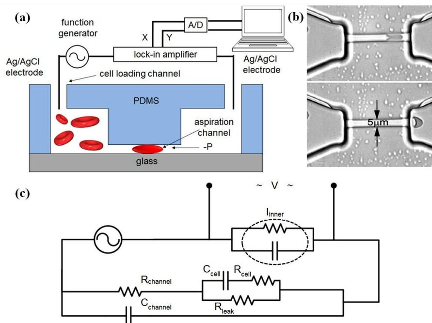
Fig. 1(a) Schematic of the microfluidic system for electrical and mechanical characterization of RBCs. (b) Measurements are made when an RBC passes through the constriction channel. (c) Equivalent circuit model of the system.
