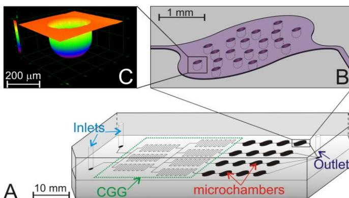
Figure 2: (A) Scheme of a microfluidic chip. (B) Microchamber (a depth of 50  $\mu\text{m}$ ). (C) Profile of a microwell (a depth of 200  $\mu\text{m}$ ,  $\text{Ø}=200 \mu\text{m}$ ).
