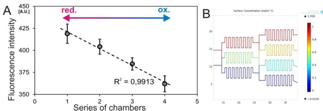
Figure 4: (A) Verification of the detection system: 1<sup>st</sup> series of microchambers contained off-chip reduced probe (highest fluorescence) and 4<sup>th</sup> series contained blank (lowest fluorescence). Fluorescence intensity in 2<sup>nd</sup> and 3<sup>rd</sup> series was in the linear range between the extremes. (B) Results of *in silico* modeling of CGG.
