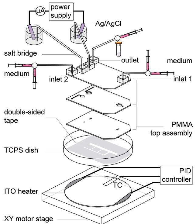
Figure 3. MFCII is composed of the PMMA top assembly, patterned double-sided tape, and the poly-styrene dish. Miniaturization of cell culture chamber in combination with an ITO heater allows easy, contamination-free cell culture and cell migration visualization. A direct current is applied through Ag/AgCl plate electrodes to introduce EF into the chip.
