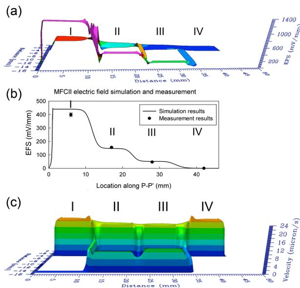
Figure 2. (a) The EF distribution of MFCII. (b) The measured EFS and simulated EFS in the middle of the 4 mm-wide channel (b) The flow field distribution in MFCII.
