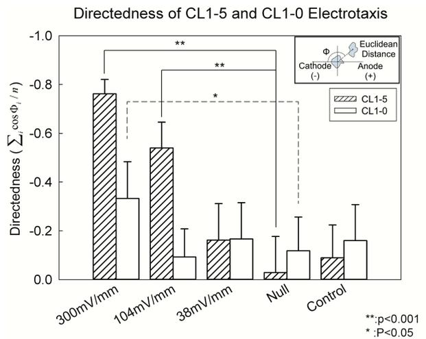
Figure 4. The directedness of CL1 cells in MFCII under three EFs, the null region in segment IV, and without electric field application as control. The inset shows the definition of directedness as average cosine of the angle between electric field vector and the Euclidean vector
