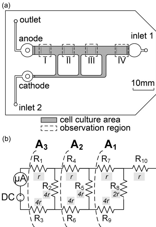
Figure 1. (a) The top view of MFCII. A 4 mm-wide channel is divided by 1 mm, 1 mm, 2 mm-wide vertical channels into segment I, II, III, IV.
