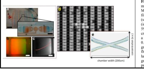
**Fig 1:** Characterization of the microjet array gradient: (a) Micrograph of the entire device filled with food-coloring dyes (scale bar = 2 mm and 0.5 mm (inset)). (b) BSA-Alexa Fluor 594 and BSA-Alexa Fluor 488 creating an opposing gradient in a single reservoir (scale bar = 0.1mm). (c) The surface gradient as visualized by fluorescein and Orange-G. (d) A large-scale 16x16 section of the gradient reservoirs. (e) Gradient profiles in the 256 reservoirs.
