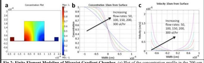
Fig 2: Finite Element Modeling of Microjet Gradient Chamber. (a) Plot of the concentration profile in the 200  $\mu$ m wide and 200  $\mu$ m tall reservoir, (b) Plots of concentration (10  $\mu$ m from the surface) at different flow-rates, (c) Plot of the velocity profile (10  $\mu$ m from the surface) at different flow rates.
