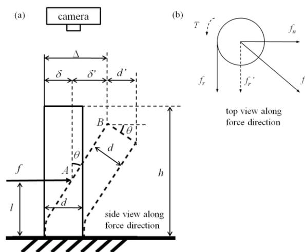
Figure 2. Schematic of the deflecting pillar model used for force analysis. (a) Measurement setup and pillar parameters. (b) Worm-pillar contact force is a composed force, i.e.  $f = f_n + f_r$ .
