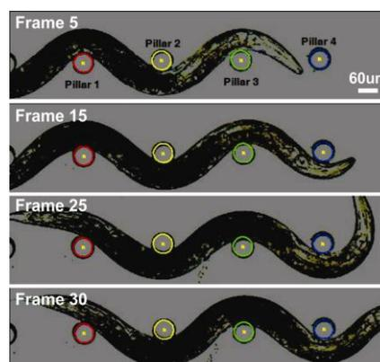
Figure 4. Micrograph sequence illustrating nematode body contact with the measurement pillars. Changes in magnitude in the force plot can be attributed to certain parts of the locomotion sequence, such as contact (Frame 5 to 15) and head bending (Frame 15-25).
