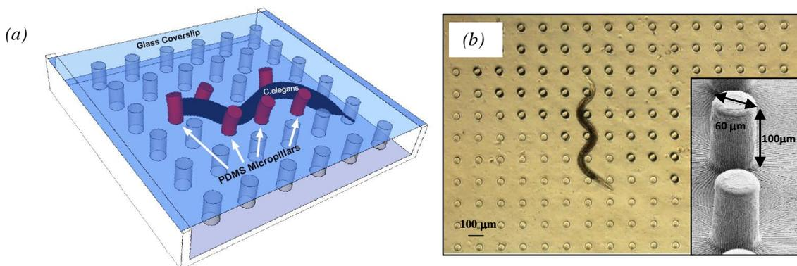
Figure 1. (a) Schematic of the *C. elegans* movement deflecting the micropillars in the PDMS device. (b) Top view of the PDMS micropillar matrix used for combined force measurement and locomotion studies. A *C. elegans* crawling inside the device in a sinusoidal movement pattern. Inset: SEM micrograph of the pillars.
