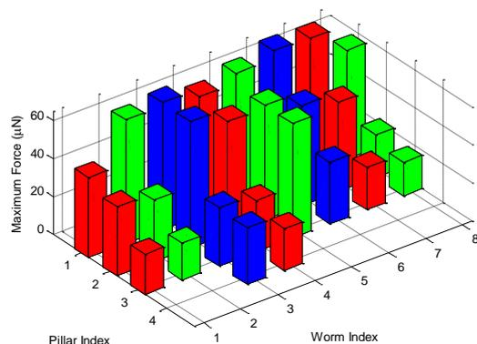
Figure 5. Maximum forces measured for eight *C. elegans*. Up to six pillars were in contact with each sample but three to four pillars bearing most forces are shown here.
