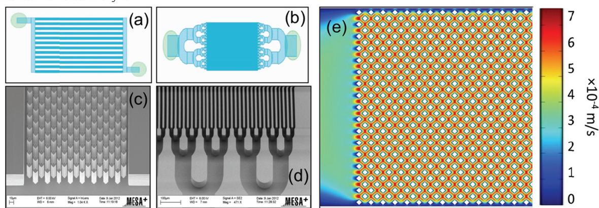
Figure 1. Chip designs and simulation. (a) straight parallel channels (b) bifurcated parallel channels (c) SEM of pillar array (d) SEM of parallel channels (e) simulated flow velocity of the pillar array.
