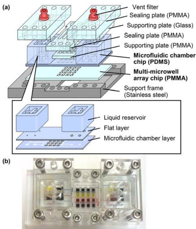
Figure 1. (a) Schematic diagrams of the microfluidic device for perfusion culture of spheroid arrays. (b) Four differently colored dye solutions were loaded into the microfluidic network on the device.
