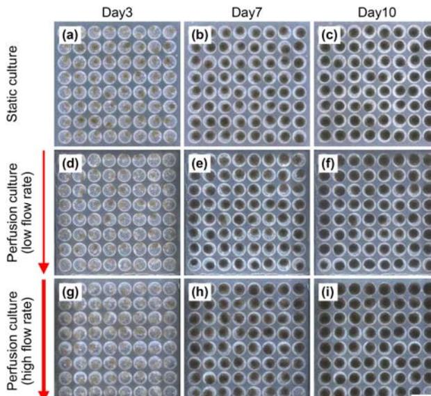
Figure 2. Phase-contrast micrographs of spheroids under static culture (a–c), low-flow-rate perfusion culture (d–f), and high-flow-rate perfusion culture (g–i). Micrographs were obtained at 3 days (a, d, g), 7 days (b, e, h), and 10 days of culture (c, f, i). Scale bar: 500  $\mu$ m.
