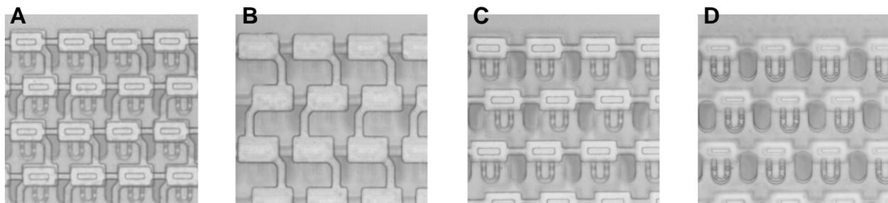
Figure 3. Microscopic images of the fabricated device. (A) An assembly showing all three layers – top and bottom pneumatic layers and a cell analysis layer. (B) Top pneumatic layer. (C) Bottom pneumatic layer. (D) Cell analysis layer.
