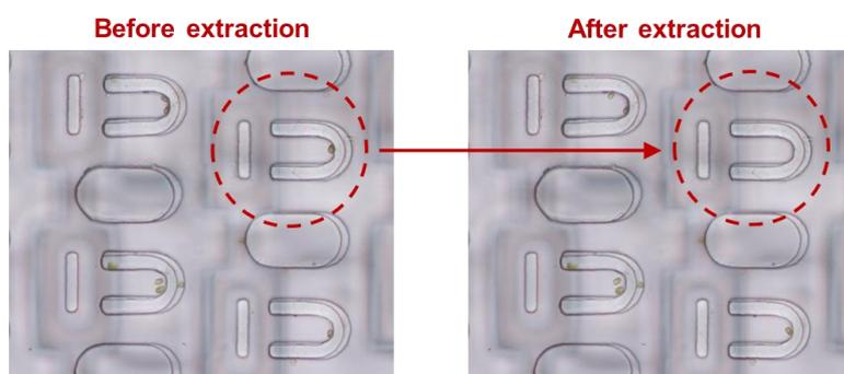
Figure 5. Microscopic images showing selective extraction of cells from the platform. *Tetraselmis suecica* cell was successfully extracted from a particular trapping site (dashed circle) without affecting cells captured at other trapping sites.
