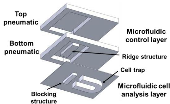
Figure 2. A schematic view of a single trapping site integrated with pneumatic control layers. Each trapping site consists of a cell trap where a single cell is captured and a blocking structure, which can be selectively opened and closed during the cell extraction process by actuating the control layers with pressure.
