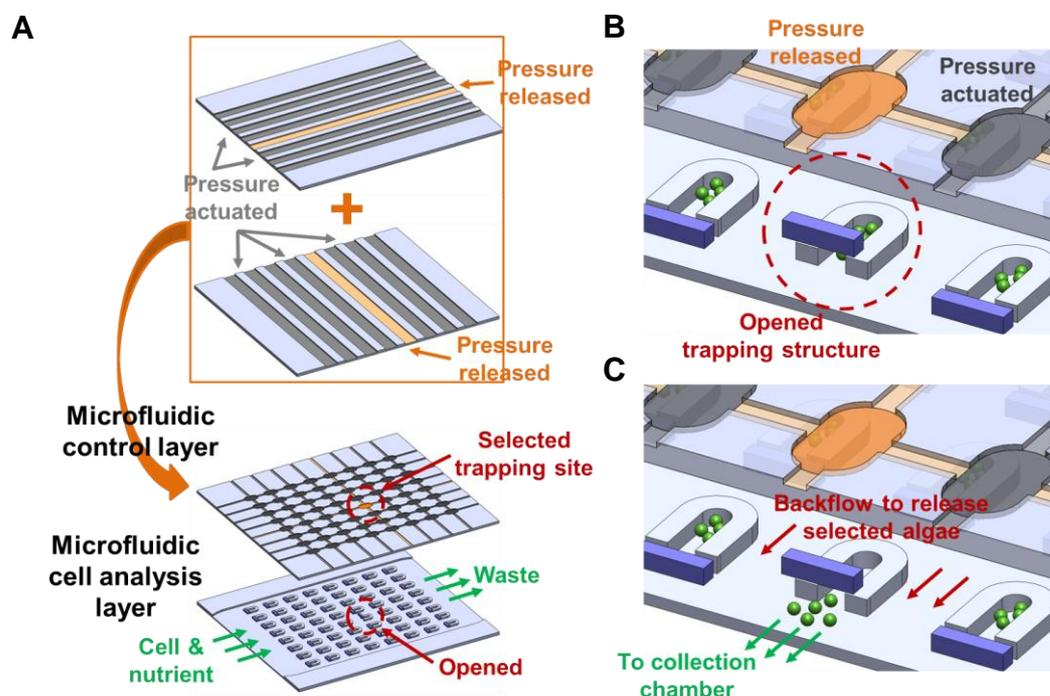
Figure 1. Illustration of a high-throughput mutagenized cell screening platform. (A) Two PDMS functional layers – a microfluidic control layer and a microfluidic cell analysis layer. (B-C) Enlarged view of a selected trapping site where both row and column channels in the control layer are released simultaneously, resulting in opened trapping site. Trapped cells can be extracted with backflow.
