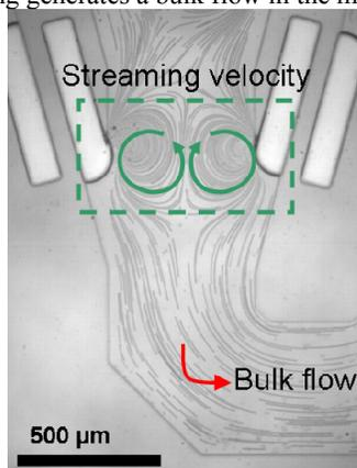
Figure 1: Streak image of ALCAT pump: Due to the angle of the ALCATs to the main channel a bulk flow is generated in addition to the acoustic microstreaming flow.
