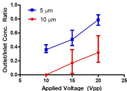
Figure 3: Characterization of particle trapping. Particle trapping decreases linearly as the applied voltage is increased. Data also demonstrates that larger particles are trapped more readily compared to smaller particles.
