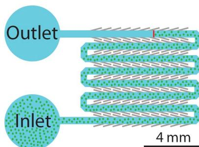
Figure 2: Design of ALCAT trapping device: Particle solution is pulled via applying vacuum to the outlet reservoir until solution arrives at the location indicated by the red line. Device is then placed on a piezoelectric transducer using ultrasound gel.
