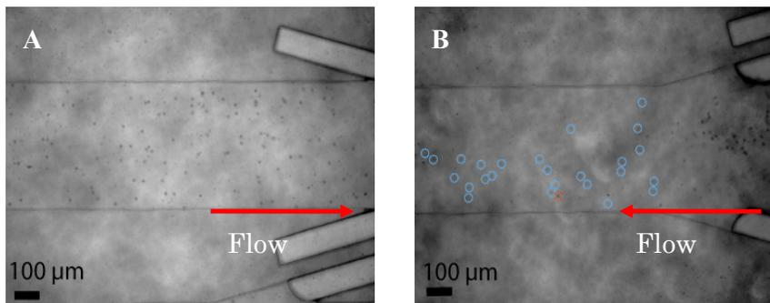
Figure 5: Micrograph of particle separation with applied voltage of 15  $V_{pp}$ . A) Inlet - Mixed population of 5  $\mu\text{m}$  and 10  $\mu\text{m}$  particles. B) Outlet - 5  $\mu\text{m}$  particles (blue circles) flow through to the outlet with a few 10  $\mu\text{m}$  particles (red circle)
