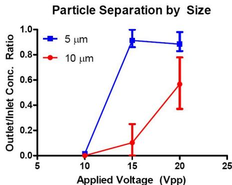
Figure 4: Results of particle separation. Smaller particles can be efficiently enriched from larger particles. Approximately a 9-fold enrichment of 5  $\mu\text{m}$  particles from a solution of 5  $\mu\text{m}$  and 10  $\mu\text{m}$  particles (1:1 ratio of concentration) can be achieved at 15  $V_{pp}$  applied voltage.
