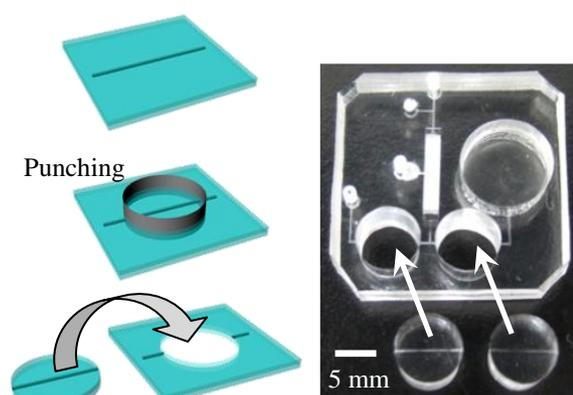
Figure 3: Fabrication process of a pair of switching valves. The PDMS residue parts in the biopsy punch after punched out were reinserted in the holes in the microfluidic chip as a pair of switching valves.
