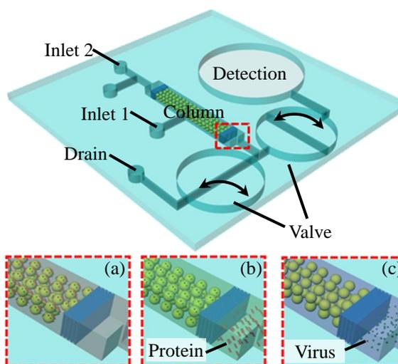
Figure 1: Concept of the microfluidic chip for on-chip hydroxyapatite chromatography.
