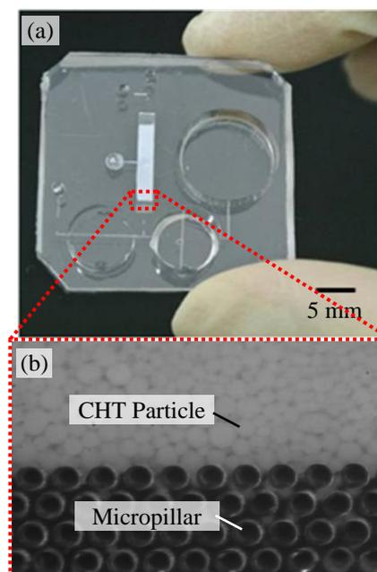
Figure 6: The fabricated microfluidic chip. CHT particles were held in the column by the cylindrical micropillars placed in the upstream and downstream part of the column.
