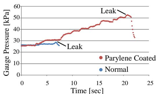
Figure 5: The results of the pressure test of the valve. The leak pressure of the valves uncoated and coated with parylene were 28.6 kPa and 52.6 kPa, respectively.
