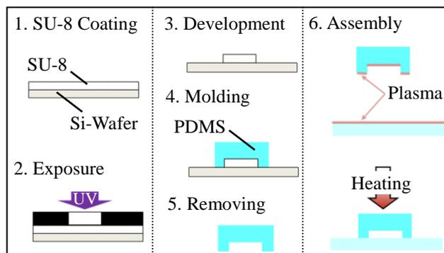
Figure 2: Fabrication process of the proposed microfluidic chip. The microfluidic chip consists of a PDMS microchannel and a PDMS substrate.
