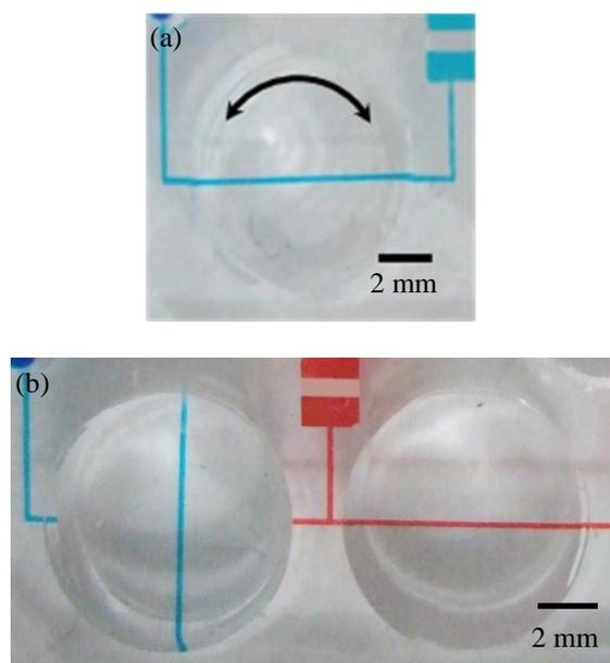
Figure 4: A pair of switching valves. The valves are opened or closed by rotation of the reinserted PDMS residue parts.
