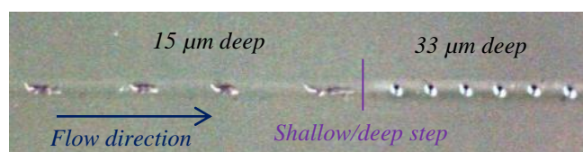
Figure 7. Droplets passing from shallow channel to the deeper channel and their reshaping.
