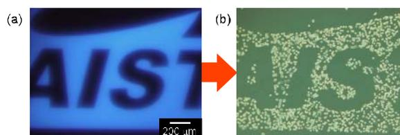
Figure 5. Cell micropatterning by micropatterned light irradiation on a cell-nonadhesive photodegradable hydrogel sheet. (a) Irradiated pattern. (b) Cells attached on the irradiated area.
