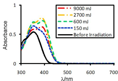
Figure 3. Absorption spectra of a 0.01 wt% solution of the photocleavable crosslinker under UV light irradiation (365 nm, 15 mW/cm<sup>2</sup>).
