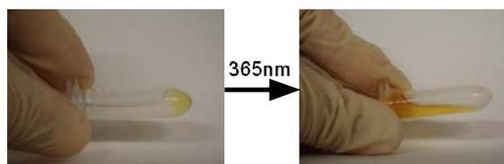
Figure 4. Degradation of the photodegradable hydrogel under UV light irradiation (365 nm, 100 mW/cm<sup>2</sup>).
