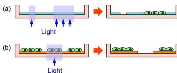
Figure 2. Schematic of optical cell manipulation on the photodegradable hydrogel sheet. (a) Cell micropatterning by means of micropatterned light irradiation on a cell-nonadhesive photodegradable hydrogel sheet. (b) Collection of target cells by means of local light irradiation on a cell-adhesive photodegradable hydrogel sheet.
