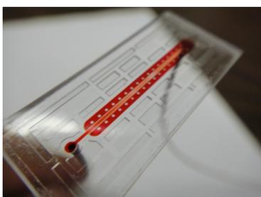
Figure 3: Sealing and leakage test of bonded microfluidic device using a red food dye diluted in water.
