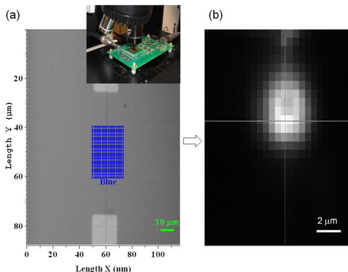
Figure 2. Raman spectral maps in the inter-electrode region (a: grid, b: integrated intensity between  $500\text{-}550\text{ cm}^{-1}$ , inset: image of the board under a confocal Raman microscope).
