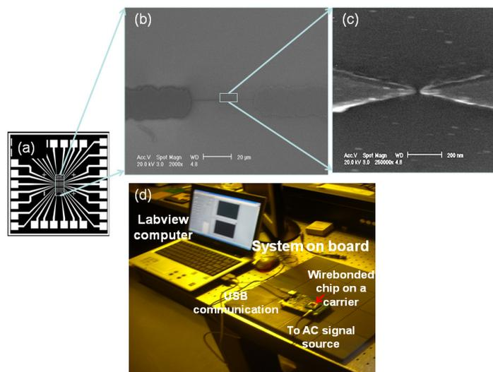
Figure 1. (a) Electrode nanogaps on a chip (scanning electron micrographs, b and c). (d) Computer-controlled integrated circuit board with field application, current amplification and data acquisition capabilities.
