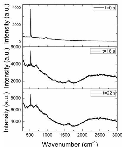
Figure 4. Time-lapse Raman spectroscopy from RPE in the vicinity of a nanogap during a trapping event. Appearance of peaks after few seconds of field application confirms protein trapping in the nanogap region.
