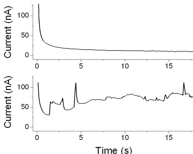
Figure 3. Negative control (upper) and electronic signature of RPE trapping across nanoelectrodes in PBS buffer (lower) with RPE concentration of 40 nM, DC bias 0.1 V, and AC signal of 1 Vpp at 1 MHz.
