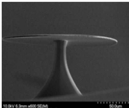
Figure 1: Scanning electron micrograph of an optical microcavity
