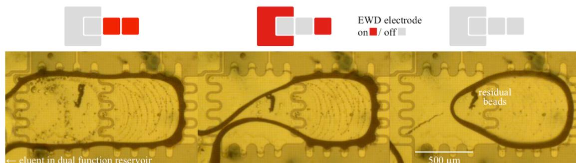
Figure 3. In this series of micrographs, an eluent droplet is dispensed from the dual function reservoir with a minimum amount of residual beads.
