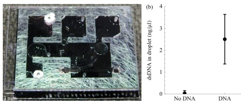
Figure 4. (a) Top-down view of the device, cf. Fig. 2a. After 60 °C elution, the GuSCN salt in lysis buffer and wash buffer 1 precipitated near the pipette ports. (b) dsDNA in the eluent droplets is determined by PicoGreen to be  $2.5 \pm 1.1$  ng/μl (95% CI,  $n = 3$ .) In the control experiments, no DNA is added during the binding step.
