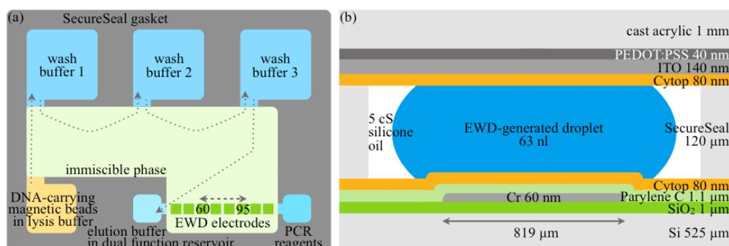
Figure 2. (a) Floor plan. Dotted line: DNA-carrying beads are transported through the preprocessor by an external magnet. Dashed line: microdrops are transported by EWD actuation. To perform PCR, an eluent microdrop mixed with PCR reagents is shuttled between the two temperature zones. (b) Device structure.
