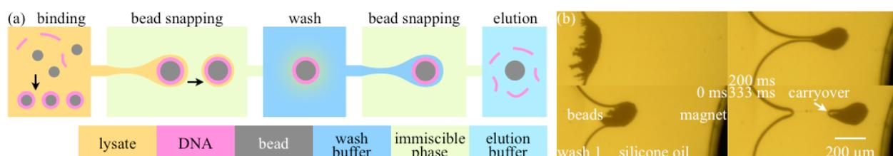
Figure 1. (a) Schematic of an immiscible phase filtration DNA preprocessor, top-down view. DNA is purified from a lysate as magnetic beads are transported through the preprocessor. (b) The sequence of micrographs shows that after wash 1 the beads were snapped from wash buffer 1 to the immiscible phase.
