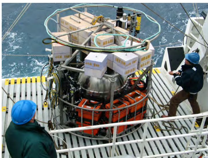
Figure 3. The ‘Deep-ESP’ being readied for a 6-day deployment to the diffuse vent field of an underwater volcano (~1600m depth). This instrument performed sandwich hybridization arrays, archivals, and qPCR with only an occasional acoustic communications-link to the ship.
